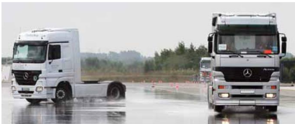
Example of control and breaking distance on a wet \mu -split surface of a vehicle equipped with ESC (Source: SAE)
