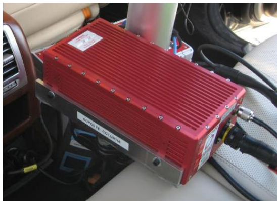
Figure 5: Installed positioning system – OXTS RT3002
