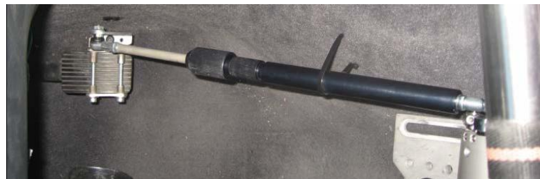
Figure 10: Accelerator robot installed in vehicle
