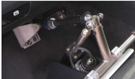
Figure 9: Braking robot installed in vehicle
