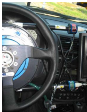
Figure 8: Steering robot installed in vehicle
