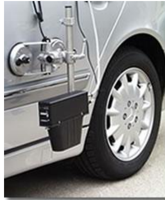
Figure 11: Optical Speed / Slip Angle Sensor
